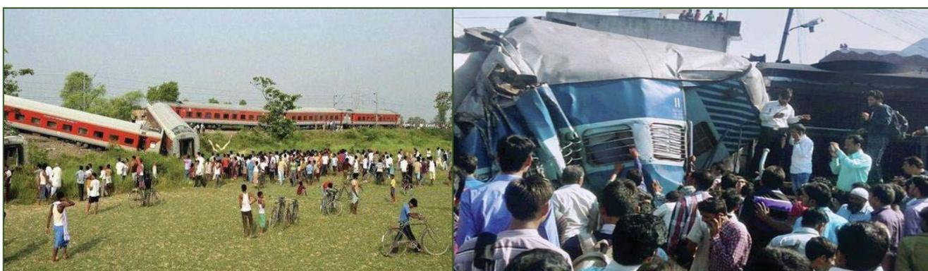
Figure 2.2: Accident site of Dibrugarh Rajdhani on 25.06.2014 - None of the LHB coaches turned turtle despite a high speed derailment and there was no loss of life (left).
